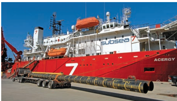
Fig. 2 Steel piles for the SSIV ready for loading to Acergy Discovery .
